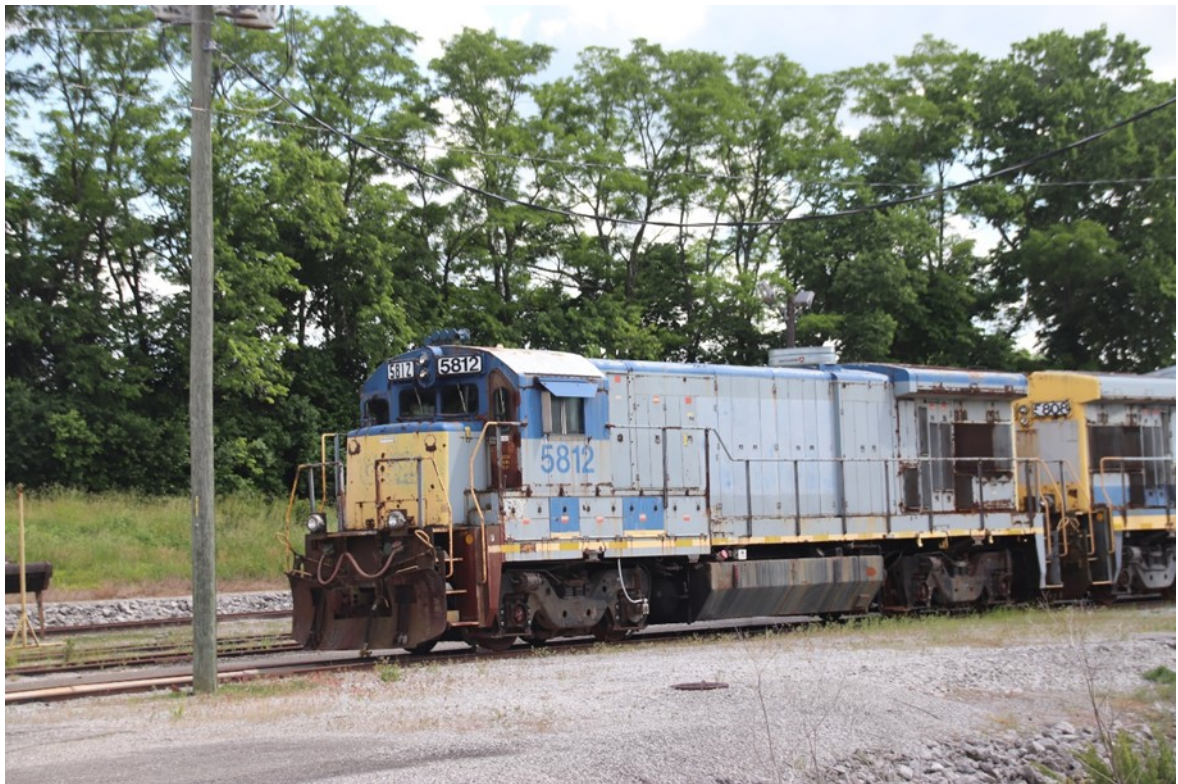
Above and below: TTI 5812 and TTI 5808, both GE B36-7 locomotives, were purchased from CSXT for use as a spare part source. Both are ex SBD
