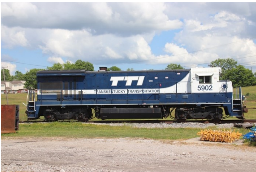
TTI 5902 a B36-7, ex CSXT, ex SBD. She is in the latest TTI paint scheme.
