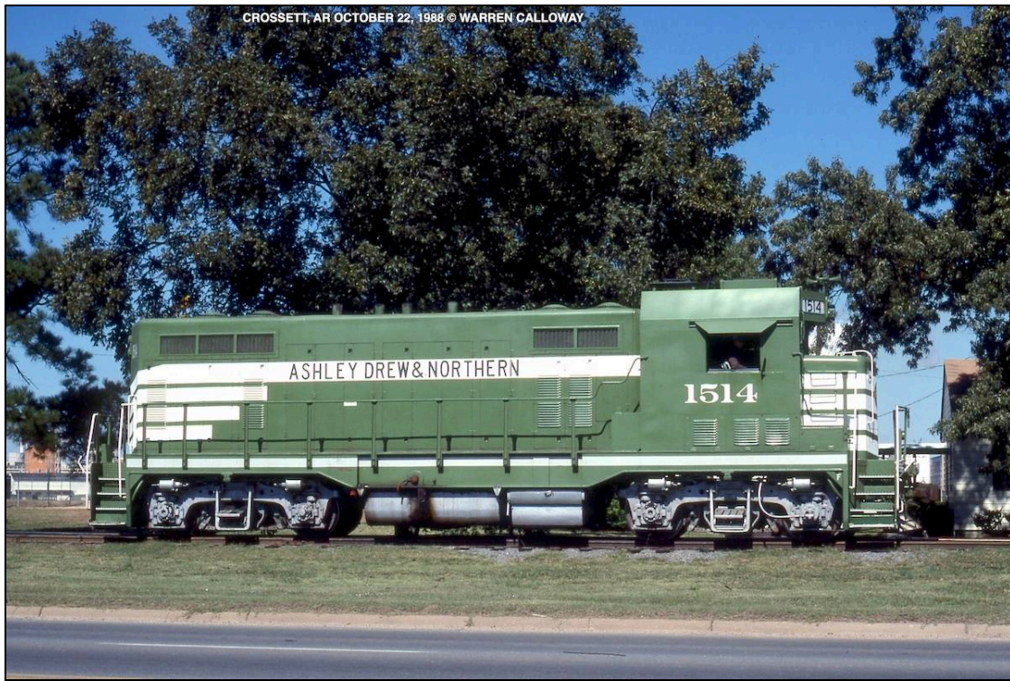
Ashley, Drew & Northern 1514 at Crossett, Arkansas on October 22, 1986. It is ex-Santa Fe CF7 2522, which was rebuilt from Santa Fe F7A 255C.
