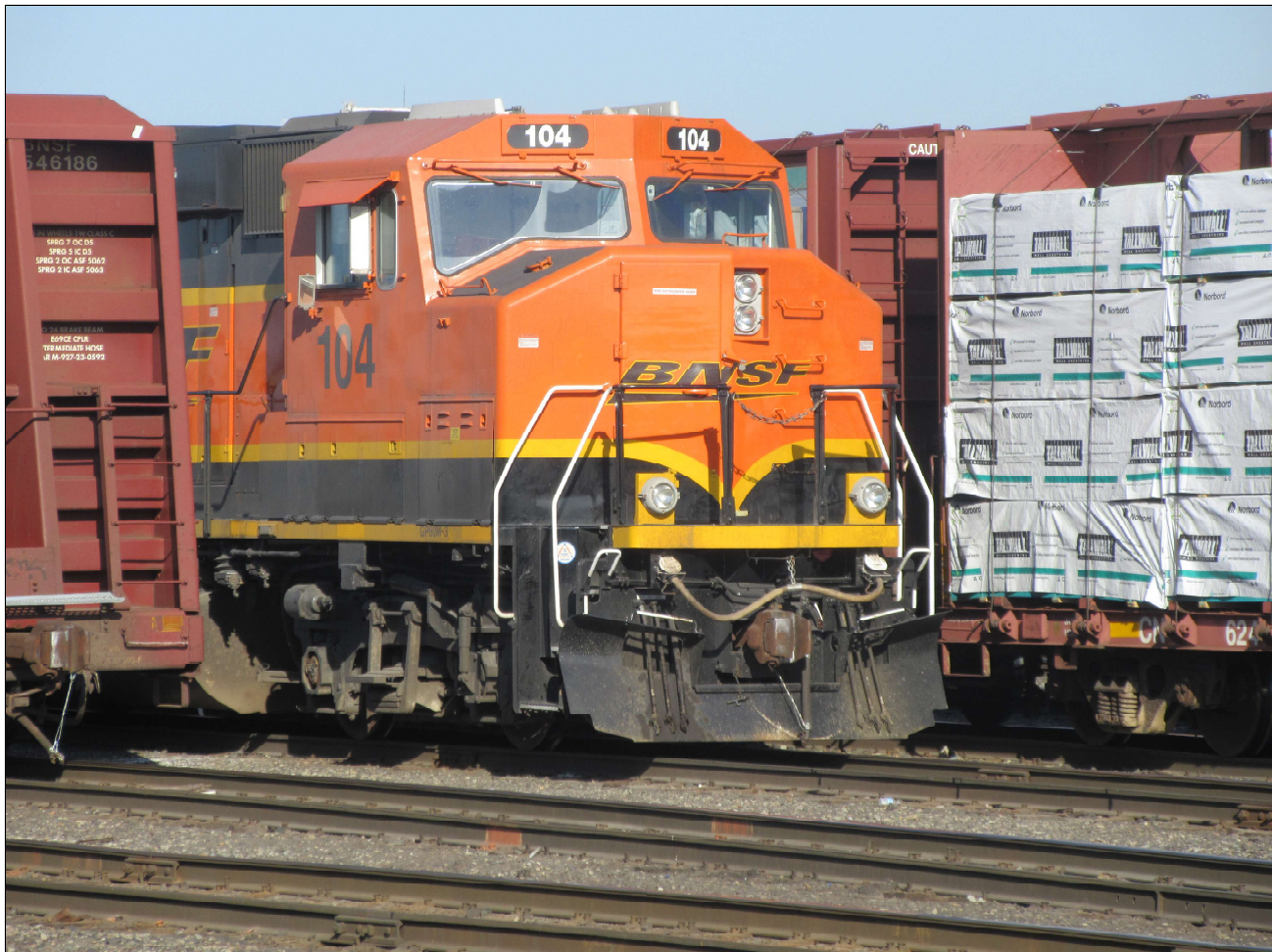
BNSF GP60M 104 peaks out between two tracks of freight cars in Spokane, Wash. on July 20, 2018. The 104 was built by EMD in July 1990 for the Santa Fe with the same number.
