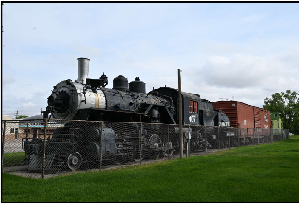
Union Pacific 2-8-0 407, nee Union Pacific 1627, built by Baldwin in 1900 on display at Legion Park in Sidney, NE along with Sidney and Lowe Railroad boxcar 10002 and Burlington Northern caboose 11357.
