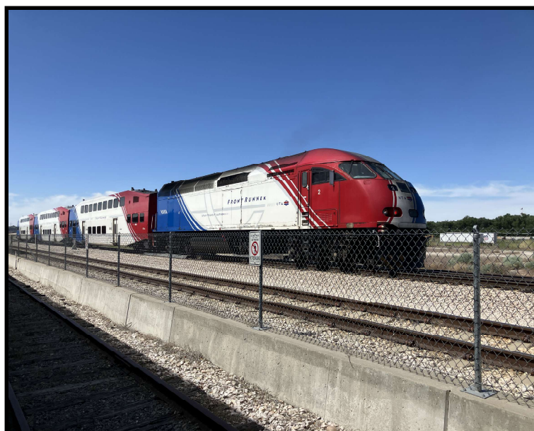
Utah Transit Authority's FrontRunner has just departed Ogden Central Station and is passing the Utah State Railroad Museum before going over the flyover as it starts the 83 mile journey to Provo. FrontRunner operates in push-pull mode; this is cab car 120 built by Bombardier and MP36PH-3C 2 built by Motive Power Industries
