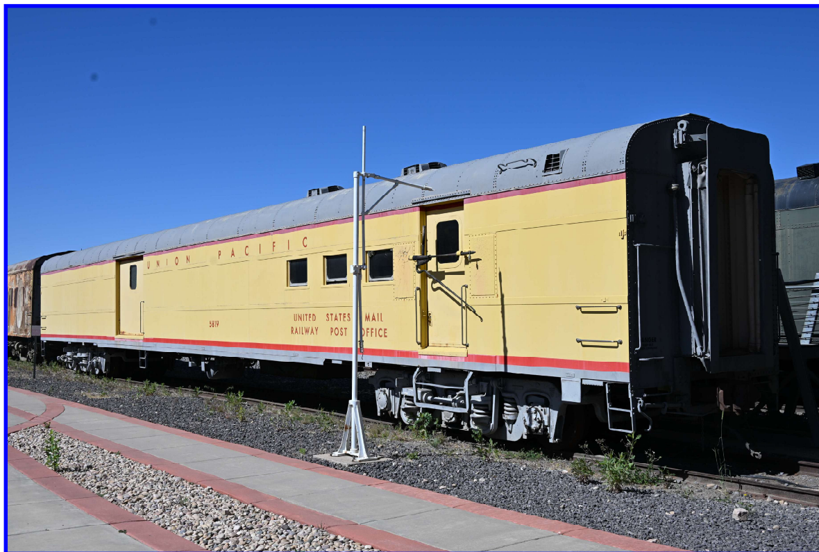
Union Pacific postal storage car 5819 built by American Car and Foundry in 1960. It saw service on the Oregon Short Line, delivering mail through southern Idaho then moved to maintenance-of-way service, becoming 903680 in 1970 and was repainted green. It has now been restored by the museum to the original yellow and gray livery with its original number.
